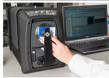
▲ A SPECTROPHOTOMETER MEASURES SPECTRAL DATA – THE AMOUNT OF LIGHT ENERGY REFLECTED FROM AN OBJECT AT SEVERAL INTERVALS ALONG THE VISIBLE SPECTRUM. THE SPECTRAL DATA IS SHOWN AS A SPECTRAL CURVE.
