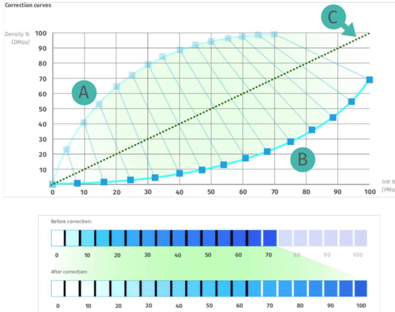
The correction curves result in linear output for a given color thus changing the behavior of the printer when the correction is applied. In the illustration to the left the results of the linearization target (A) are mapped to the corresponding correction curve (B) in order to achieve linear behavior of the device (C).
